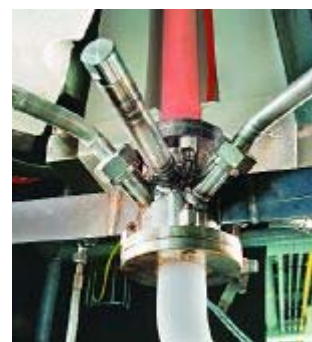
REACTOR At Degussa Advanced Nanomaterials' Hanau, Germany, site, this hot-wall reactor is used in the R&D department for process development. DEGUSSA ADVANCED NANOMATERIALS
